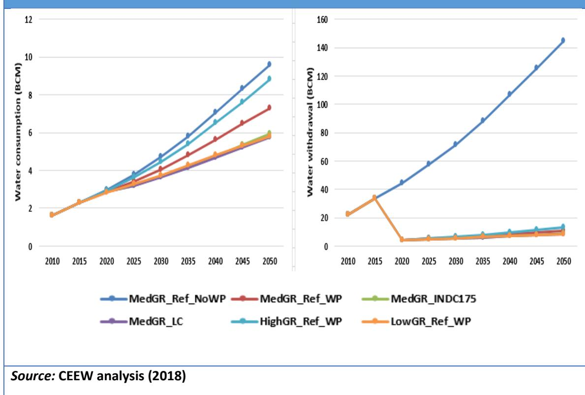
There is some interesting dynamics that need to be highlighted- when older plants move from OTC to CT technology, there is an increase in water consumption. The consumption coefficient of CT technology is higher as compared to the OTC technology. But all the new power plants, have to adhere
